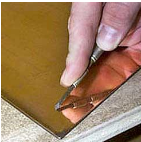
Prior to photo-engraving printing plates were etched by hand
